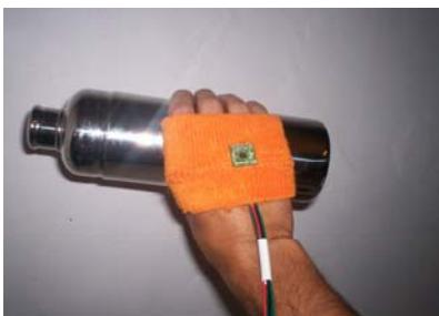
Figure 6. Accelerometer woven into a textile band.
